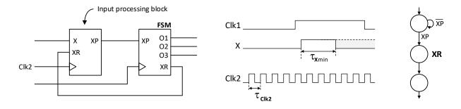
(16 points) Sketch a state diagram for the input processing block that meets all the requirements.
