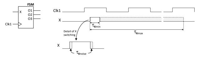
You decide to add an input processing block that uses a new clock (Clk2) that has a period less than  $\tau_{Xmin}$  but greater than time  $\tau_{Xnoise}$  (Clk2 can be used to sample X, because at least one rising edge will occur during the time X is asserted, and it will filter out the logic/switching noise). But because  $\tau_{Xmax}$  isn't specified, there could be any number of rising edges on Clk2 during the time X is asserted.
