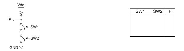
The example circuit below asserts its output as a logic 1 when either switch is closed. Sketch a new circuit that asserts logic 0 whenever one or both switches are closed. Label the switches 1 and 2, and complete the truth table below. Circle the correct term (high or low, and open or closed) to complete the following sentences describing the AND and OR relationships for your circuit:
