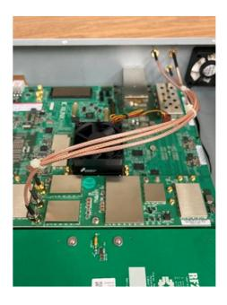
**22.** Install 2 right angle connector header (#12) to PMOD cables (#7). Install the PMOD cables to ZCU216 and RF216 Main board as shown below. Pay particular attention to pin 1 markings on cables and pin 1 markings on pc boards.
