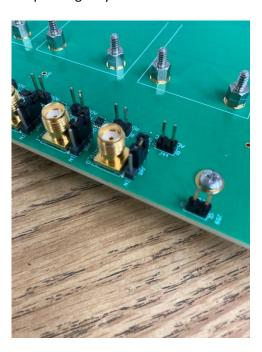
**6.** Connect the RF216 Main board to the ZCU216 board, and use the ZCU216's jackscrews to secure the boards together as shown.
