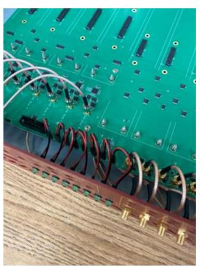
14. Install the panel mount side of IDC Cable (#8) in rectangular cutout marked "USER I/O" on the enclosure front panel, with the tab cutout side of connector facing up. Use ½" 4-40 screws (#20) and 4-40 nuts (#21) to secure header to front panel. Insert opposite end of IDC Cable in connector J60 on RF216 Main board. Match pin 1 of cable connector with J60 connector pin 1 designator.
