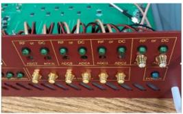
17. Insert eight 6" LEDs (#3) in enclosure front panel holes labeled "RF" and "DC" above the "DAC" SMAs. Connect other end of the eight 6" LEDs to the eight 2-pin headers labeled "DACxx\_RF" and "DACxx\_DC" on the RF216 Main board. The "xx" value of the 2-pin header should match the value of the associated DAC SMA cables. Notice that the 2-pin header has one pin labeled "B"
