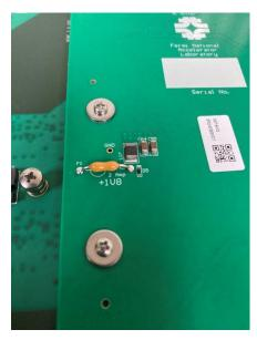
**7.** Place ZCU216/RF216 Main board assembly in the enclosure with ZCU216 toward rear of enclosure. Secure the board assembly to enclosure using 10 screws (#14) for RF216 Main board, and the screws provided with ZCU216 to attach the ZCU216 board. Mounting holes are pre-drilled in the enclosure.
