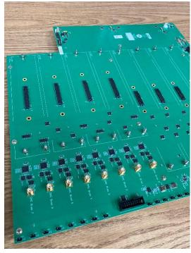
**5.** Using small needle nose pliers (or fingers), install 6 shunt jumpers (#19) on USERIO 0-5 3-pin headers as shown below. Choose IN or OUT depending on your needs.
