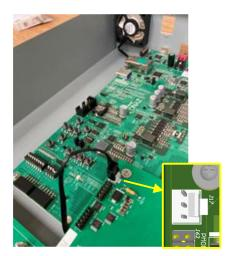
**9.** Install right fan (#10) using 4 screws provided with the fan. Note the orientation of the fan plug wire and the direction the fan is facing. Connect right fan to RF216 Main board at connector J16.
