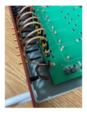
**16.** Insert as many 15" SMA cables as necessary for your "OUT" and "IN" daughter board configuration into enclosure front panel holes labeled "DACx" and/or "ADCx". "DAC" (Or "OUT" daughter boards) use 4 SMA cables each, and "ADC" (Or "IN" daughter boards) use 2 SMA cables each. Note that daughterboard cables ship with the daughterboards.
