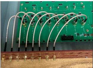
**12.** Install six 7" SMA cables (#5) in the "USER I/O" 0-5 labeled front panel holes. Use the SMA torque wrench to install opposite end of "USER I/O" SMA cables on "USER I/O" SMA connectors on RF216 Main board.
