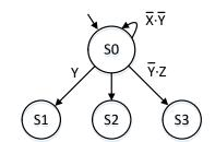
5. (7 points) The figure shows a state machine with outputs going to various destinations. Circle the letter of any output that should have logic noise (glitches) removed.
