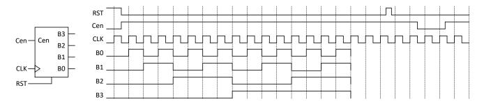
**2.** (12 points) Complete the circuit sketch for a four-bit synchronous binary counter by adding the required next-state logic gates in front of the flip-flops. (Hint: you can possibly sketch a circuit directly by observing that each more significant bit changes state when all the previous bits are a '1', or you can create K-maps and loop out minimum circuits... watch for XOR's)!
