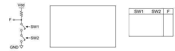
The example circuit below asserts its output as Vdd when either switch is closed. Sketch a new circuit in the box below that asserts F as GND whenever one or both switches are closed. Label the switches 1 and 2, and complete the truth table below. Circle the correct term (high or low, and open or closed) to complete the following sentences describing the AND and OR relationships for your new circuit.
